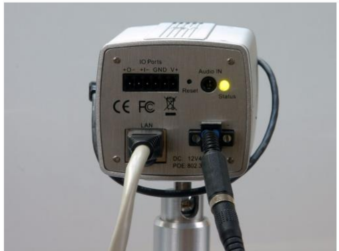
lug in the 12V DC connector to the power plug converter
