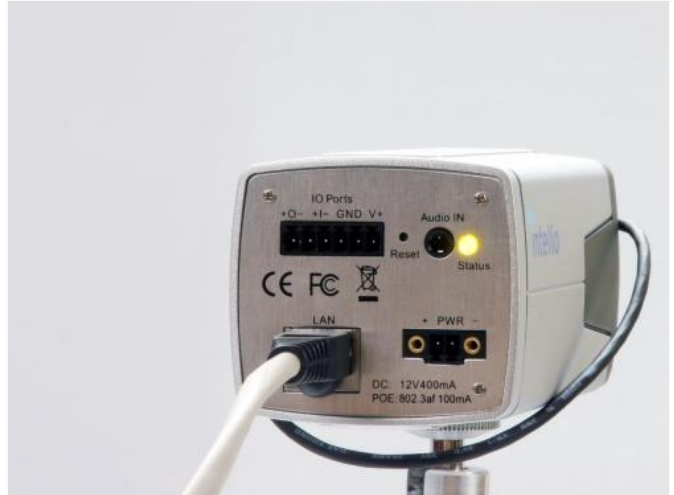
The status LED is green, the camera is powered and has IP address
