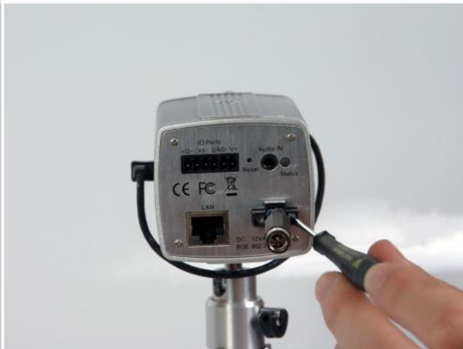
Assamble the power plug converted
