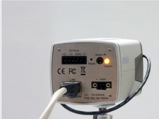
The status LED is yellow, the camera is powered
