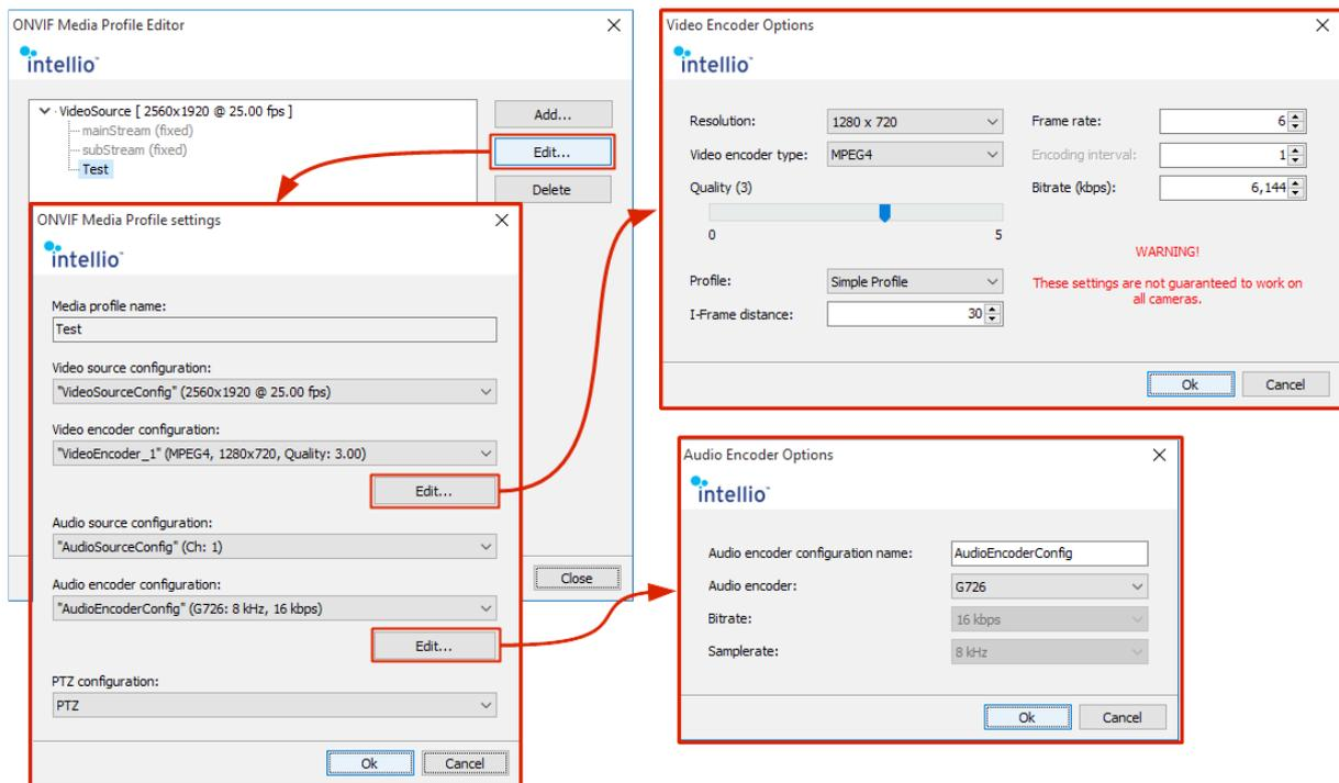
**I-Frame distance:** The IVS4 software requires a distance of maximum 50 frames between I-frames transmitted by the camera (*the ideal number of frames is maximum 30*). This causes no problems in most cases; however with default setting this value can be considerably higher for cameras of certain manufacturers (*e.g. Panasonic, Bosch*).
